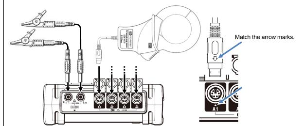
Number of clamp sensors to be used varies depending on the wiring configuration under test. See "Wiring diagrams" (P.37) in this manual.
