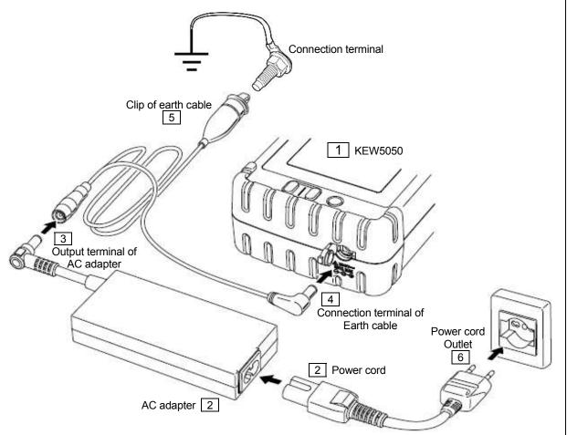
The Product can derive power from a measurement line of 240 V or less to ground by using an optional power adapter, MODEL8329. For further detail, see "9.3 Getting power from measured line" (P. 78).
