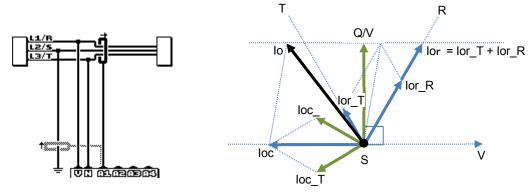
In the above illustration, lor\_R and lor\_T represent resistive leakage current in R and T phase, and loc\_R and loc\_T represent capacitive leakage current in R and T phase respectively.
