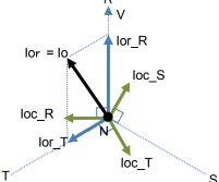
The vector direction of **lo** helps to identify the phase with relevant degraded insulation.
