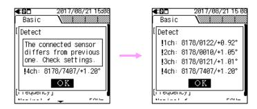
Manual configuration is required for general purpose leakage clamp sensor or load current clamp sensor; the settings aren't updated automatically.
