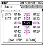
If the display of the selectable items is like the one shown to the left, the highlighted cursor can move to up, down, right and left. Use keys and select the sensor to be connected, and then press (ENTER) to confirm. To return to the previous screen and cancel the changes, press the (ESC)
