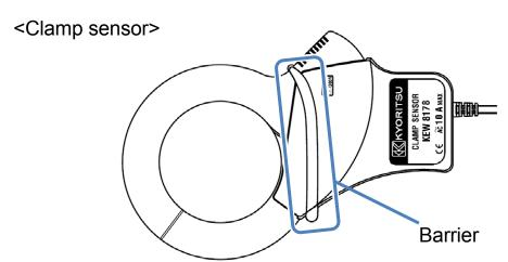
Barrier is a mechanical safety part and provides protection against electrical shock and ensures the minimum required air and creepage distances. Keep your fingers and hands behind the barrier during a measurement.
